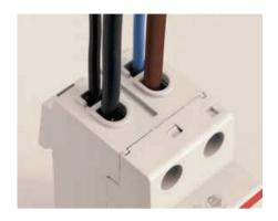
Two terminals are available, the fore one for cables up to 25 mm<sup>2</sup>, the back one for cables up to 10 mm<sup>2</sup> or for busbars.
